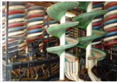
Spiral section on Dredge DI's wet separation plant
